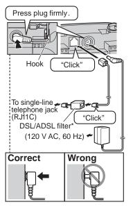
\*DSL/ADSL filter (not supplied) is required if you have DSL/ADSL service.
